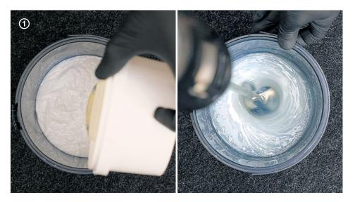
$\rightarrow$  Pour part B following the catalysis ratio Part A : Part B = 2 : 1 (by weight).
