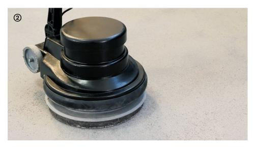
→ Cement-based substrates must be suitably sanded (diamond disc/ carborundum/36 grain sandpaper).
