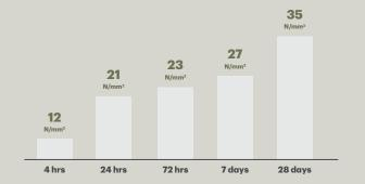
Planogel Rheo ensures high compressive strength after only a few hours, making it suitable for laying ceramic tiles from the very beginning.
