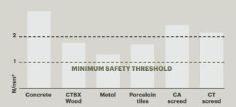
Planogel Rheo's adhesion on different types of substrates, suitably prepared and treated with suitable primers.
