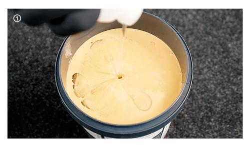
→ Before use, stir part A, add the hardening compound whilst stirring in the ratio part A: part B = 5:1. Mix well, then dilute 10% using clean water and mix again.
