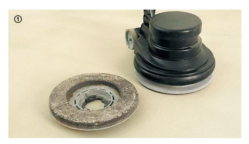
→ The **Floorzero** layer must be carefully prepared. Collect the excess quartz, then sand with a mechanical buffer (carborundum disk, followed by 36 grain) and thoroughly vacuum to remove any sanding residue.
